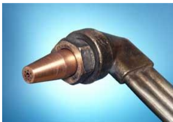
Figure 4. Standard nozzle with central bore for oxygen jet and a ring of ports preheat gas mixture
