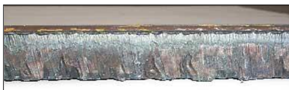
Figure 7. Too high plate nozzle to plate distance
