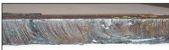
Figure 8. Too High Oxygen Flow
